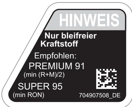
1000R-MOTOREN - IN DER NÄHE DES KRAFTSTOFFTANKDECKELS
