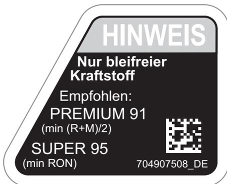
**1000R-MOTOREN - IN DER NÄHE DES KRAFTSTOFFTANKDECKELS**
