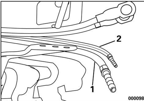
1. Flexible et raccord de carburant – 9 mm (3/8 po)
