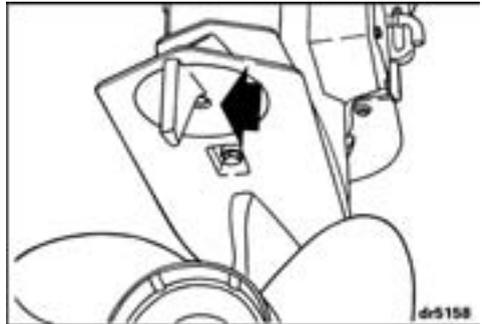
Tighten the trim tab screw to a torque of 11 to 15 ft. lbs. (15 to 20 N-m).
