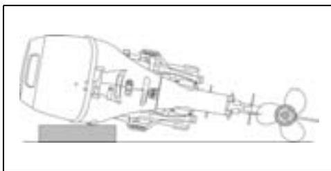
**IMPORTANT:** Do not let the gearcase of the outboard sit higher than the powerhead during transporting or storing. Water may drain into the powerhead, causing damage to the engine.
