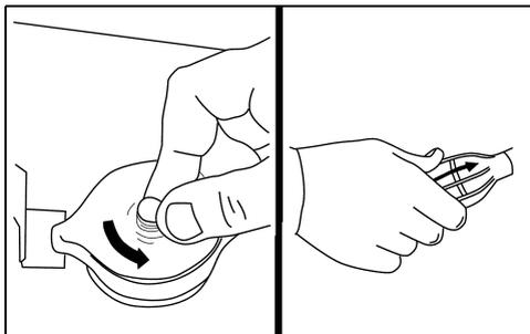
Connect the clip to the emergency stop/key switch. Snap the lanyard to a **secure** place on the operator's clothing or life vest — not where it might tear away instead of activating the stop switch.
