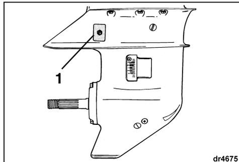
1. Anode anticorrosion
