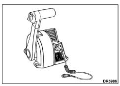
**IMPORTANT:** When shifting from FORWARD to REVERSE or from REVERSE to FORWARD, pause at NEUTRAL until the engine is at idle speed and the boat has slowed.
