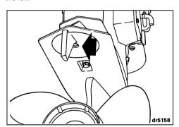
Tighten the trim tab screw to a torque of 35 to 40 ft. lbs. (47 to 54  $N \cdot m$ ).
