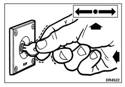
**IMPORTANT:** The starter motor can be damaged if operated continuously for more than 10 seconds.
