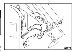
**To disengage bracket** — Tilt the motor fully. Return the trailering bracket to its stowed position. Lower the motor to its vertical position.
