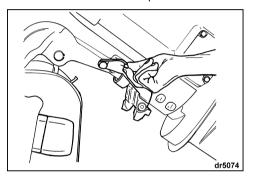
Trailer your boat with the motor in a vertical position. If your trailer does not provide adequate road clearance, the motor can be trailered while tilted by using the motor's trailering bracket.
