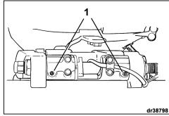
Tilt tube lubrication points.
