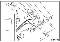
1. Trailering bracket lubrication points.
