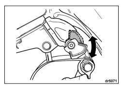
Disengage the tilt support lever:
