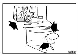
Galvanic corrosion destroys underwater metal parts and can occur in fresh or salt water; however, salt, brackish and polluted waters will accelerate corrosion.
