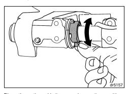
Place the outboard in its normal operating position. Rotate the tilt limiter cam — pull its tab forward and up to REDUCE the amount of tilt UP.
