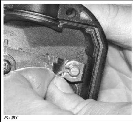
Detach throttle body side cover from throttle body.
