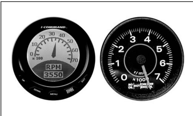
Typical *I-Command* and *SystemCheck* gauges 007988
