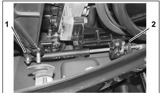
1. Shift cable retainer clip and washer
