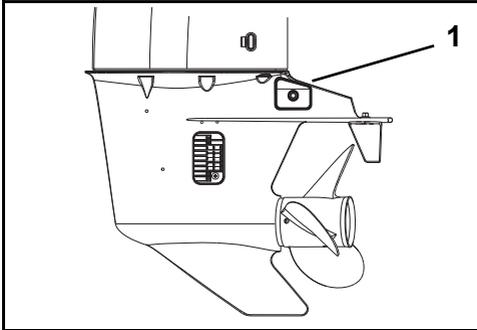
1. Anti-corrosion anode
