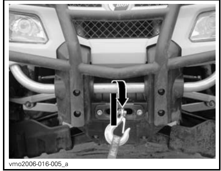
TYPICAL — FRONT TIE-DOWN POINT LOCATION
