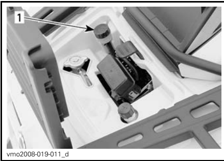
TYPICAL — SERVICE COMPARTMENT 1. Reservoir
